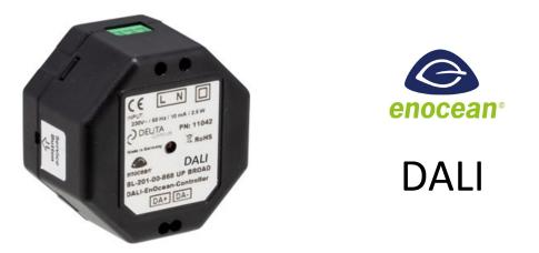
The EnOcean DALI controller type **BL-201-00-868 UP BROADCAST** offers a DALI master and an integrated DALI power supply unit for the direct connection of up to 17 slaves (lout max. = 34 mA) without the need for a separate DALI power supply unit.
