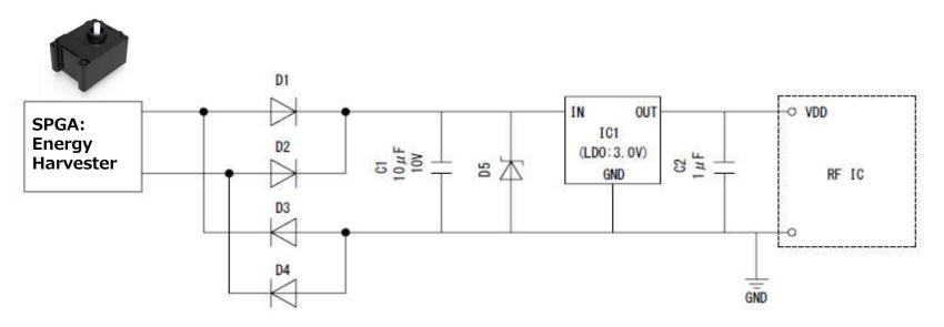
SPGA generates reverse polarity electric generation when you "press" and "release" the device.
