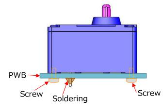
Please use this product attached to PWB. Please should be installed this product by not only soldering the terminal but also putting screw to the boss hole when you Install this product.
