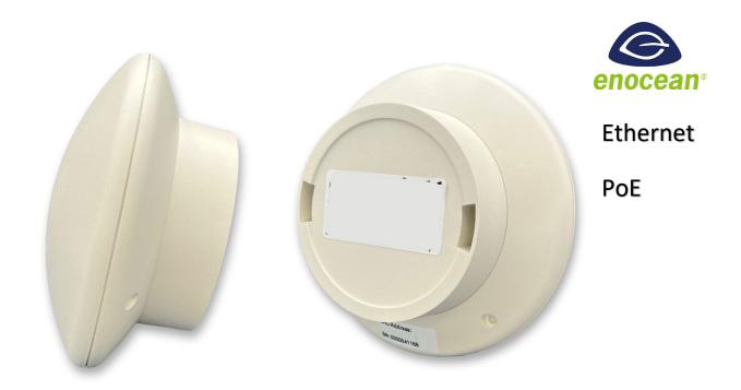
The IP-EnOcean-Bridge **AL-512-00-921 white / EnoDisc®** provides an Ethernet interface and an EnOcean transceiver, to receive EnOcean sensor data via 921,7 MHz, and to transmit data to actuators and configuration data via the wireless EnOcean interface.
